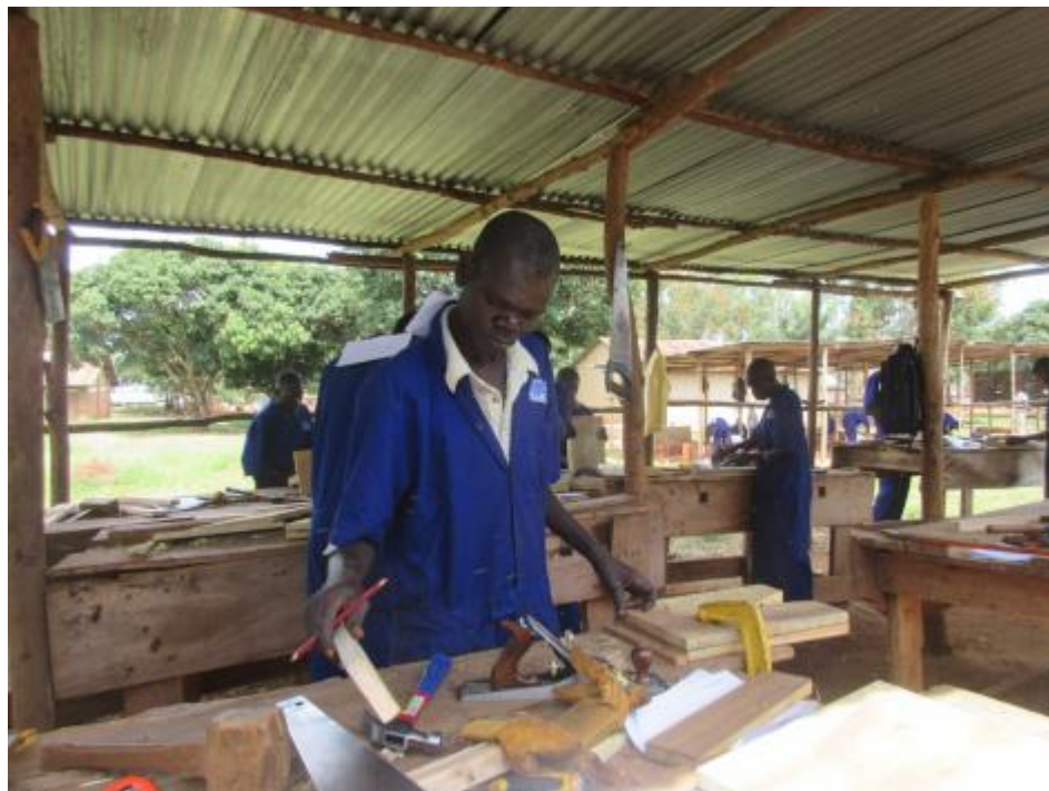
A Carpentry and Joinery student makes a stool according to the plans provided
